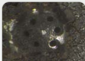
GDI fuel injector nozzle tip with coked deposits, after 24 hr Clean-Up (CU) test phase.
