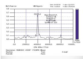
200 HP Roots Blower at a chemical plant is experiencing high vibrations while being lubricated with a competitor's ISO 320 EP gear oil.
